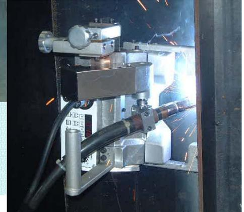
Light, compact, 4WD, and magnetic force traction with low center of gravity achieves highest pulling power and stability in the market.
