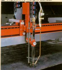
In order to keep a constant distance in between the tip and the plate during cutting (necessary for quality cutting) an electrostatic capacitive height adjustment system can be mounted.
