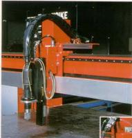
cutting has become reality by adding linear guide ways and slides to the X-direction main drive carriage and sub carriages.
