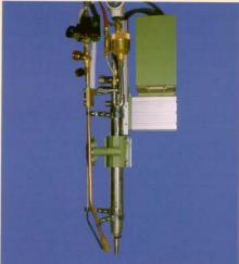
To mark lines on the steel plate (for welding or bending purposes) it is ideal to use a powdermarkng unit.
