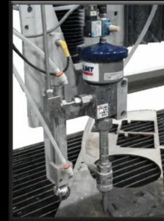
**IDE™ II Abrasive Waterjet Cutting Head**
